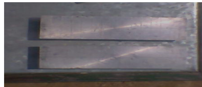
Figure 4: Stir casted Al6063/15% SiCp MMCs after machining.
