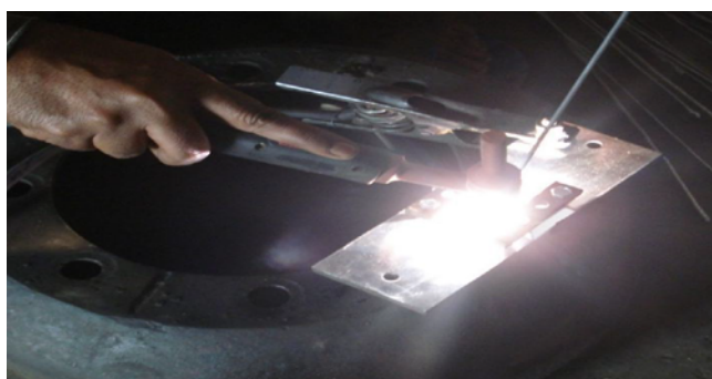
Figure 5: Joining of MMCs work specimen.
