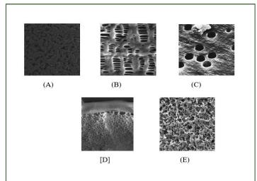
**Figure 2:** Morphology (SEM image): A) Sintering, B) Stretching, C) Track-etching, D) Solution coatings (cross section of a composite membrane and E) Phase inversion.
