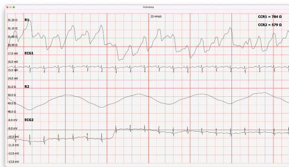
Figure 4: The result of the base impedance after light physical activity is \approx 31.0 Ohm in the volunteer of the “Control” group (R1 - base impedance, ECG - ECG signal, R2 - breathing pattern).
