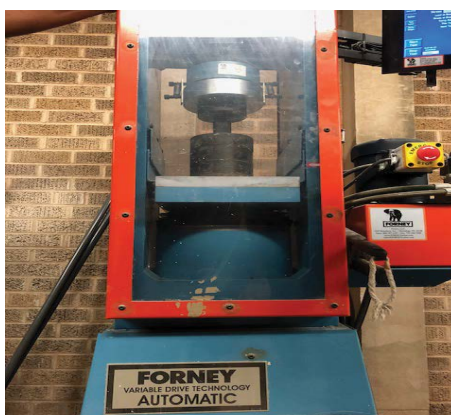
Figure 1: Compressive strength machine used in fracturing the samples.
