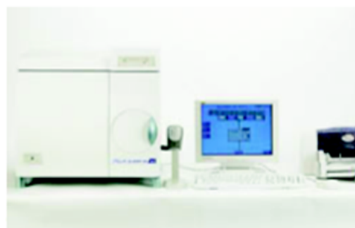
Figure 1: The Bact/ALERT.3D microbial detection system based on patented colorimetric sensor-and-detection technology for tracking CO 2 production. ( www.biomerieux-usa.com ).
