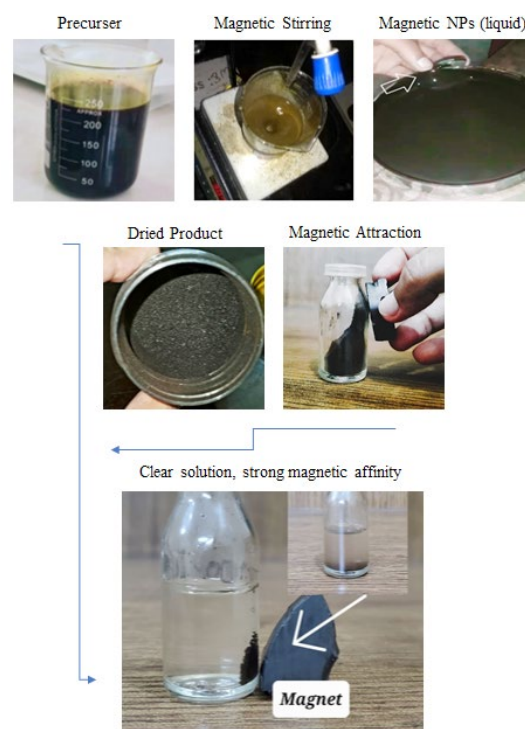
Figure-2. Chemical synthesis for Magnetic nanoparticles.
