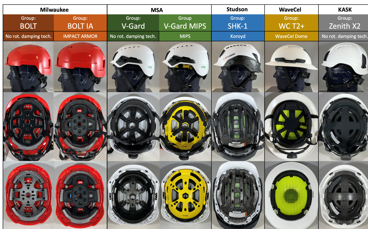
Figure 2: Seven Type II-rated helmets, four of which had a dedicated rotation damping technology. The third row of images depicts inside views of helmets after removing the comfort liner, fit system, and chin strap to better visualize the impact liner.
