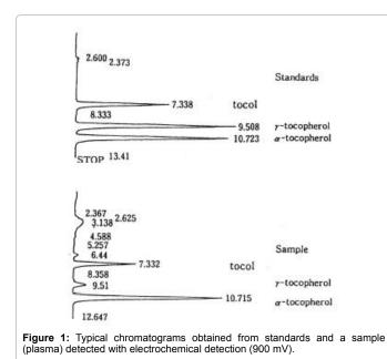
equipped with 250 mm×4 mm i.d. RP-18 column (Shiseido Co., Sepak C-18). The mobile phase was 100:2:7 (v/v/w) methanol:H<sub>2</sub>O:NaClO<sub>2</sub> at 1 ml/min. The injection volume was 10  $\mu$ L. Typical chromatograms detected by ECD 900 mV are illustrated in figure 1.
