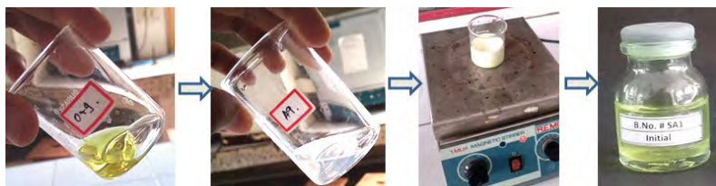
Figure 1: Preparation of polymeric micelles by using solvent emulsification method.
